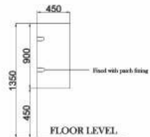
ELEVATION OF URINAL PARTITION (Unit in mm)
