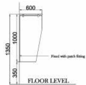
ELEVATION OF URINAL PARTITION (Unit in mm)
